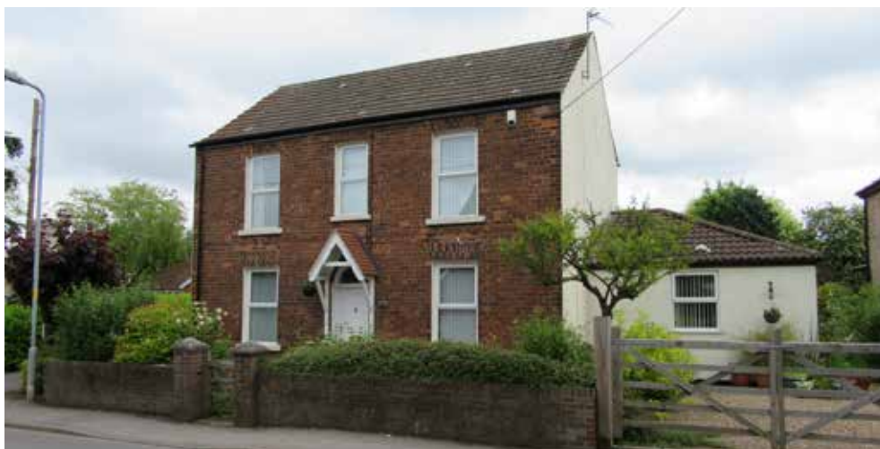
Fig 184: 111 High Street, like many of the other vernacular properties in this part of Scotter, displays a red brickwork facade but also has areas of cream-coloured render, whilst windows and doors are arranged to achieve symmetry within the facade
