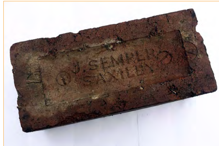
Figure 2.4: Photo of old Saxilby brick, frequently used in the older building stock (Source: Saxilby & District History Group).
